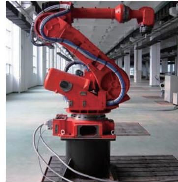
Figure 2. SRD165A spot-welding robot
