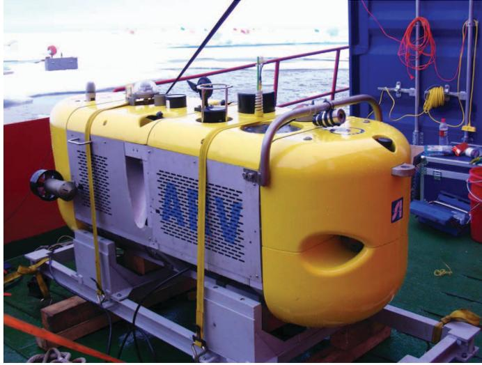
Fig.1 ARV on its support vessel
