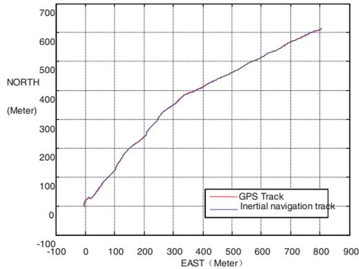
Fig.5. Inertial Navigation tracks and GPS tracks
