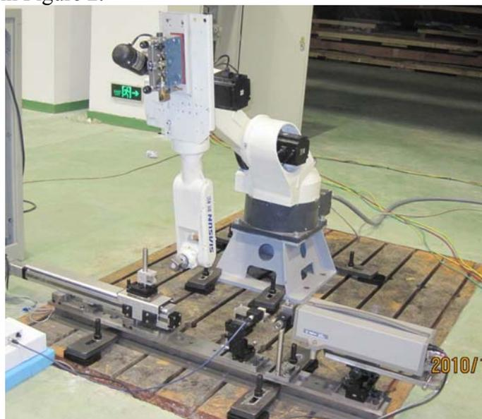
Fig. 2. Laser tracking measurement system
