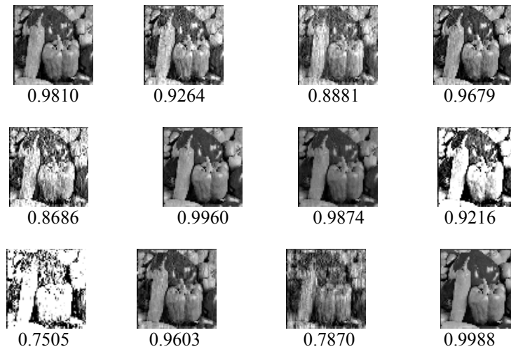
Fig 4 The best extracted watermark under different attacks and their corresponding correlation coefficients.
