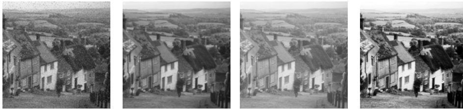
Salt & pepper noise 0.04 mean filter 3 gamma correction histogram eq
