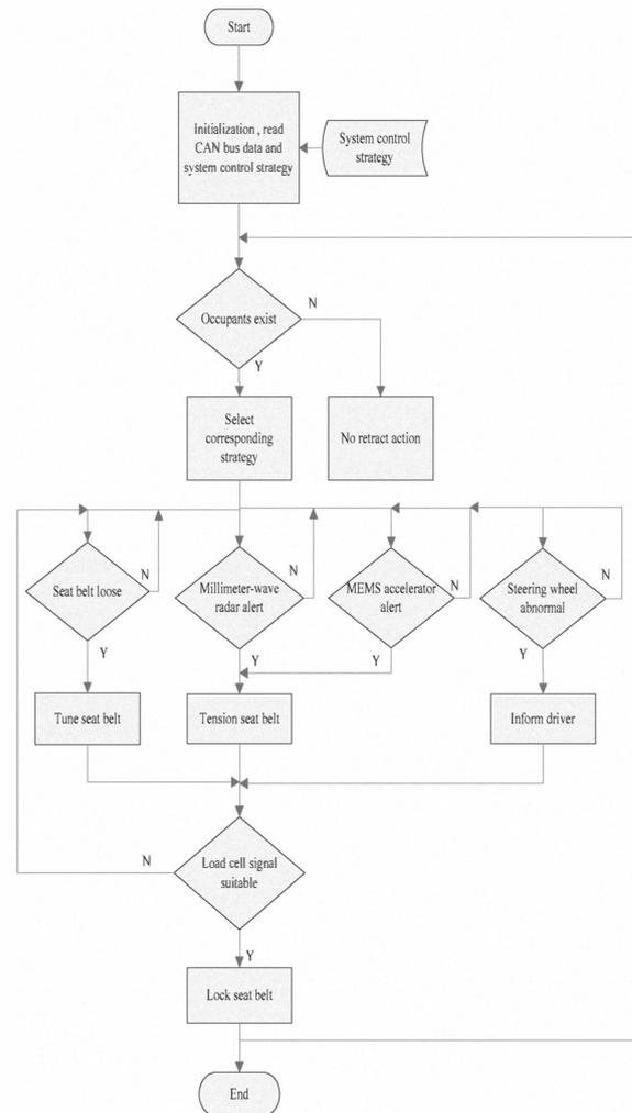
Figure 3. Active control seat belt retractor control program flow
