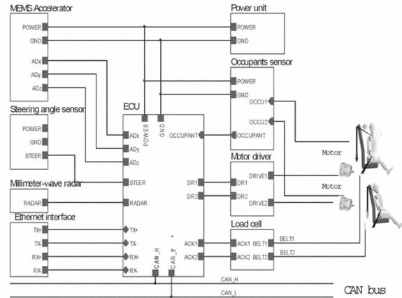
Figure 2. Electronic seat belt retractor control system schematics
