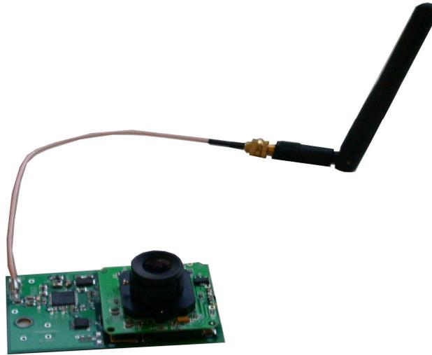
Fig.3 wireless video sensor networks node
