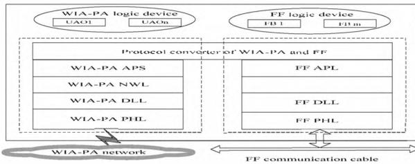
Figure 4. Architecture of WIA-PA and FF interoperation gateway
