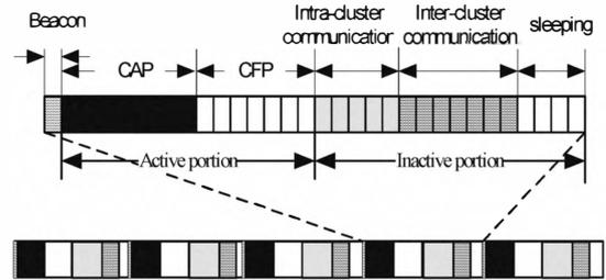
Figure 2. Structure of WIA-PA MAC layer superframe
