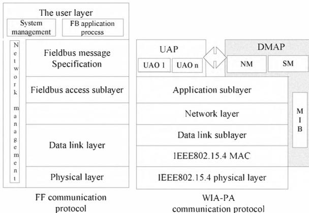
Figure 1. WIA-PA and FF communication protocol model
