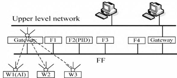
Figure 5. A simple example of hybrid WIA-PA and FF field network
