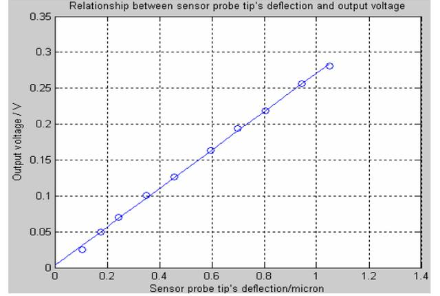
Fig. 5 The curve of relationship between the deflection and the output voltage of signal processing circuit.
