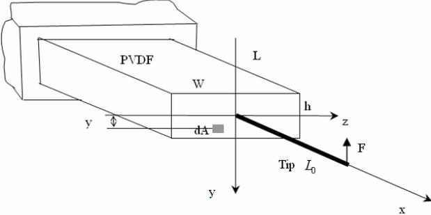
Fig. 1 The schematic diagram of the micro-force sensor.
