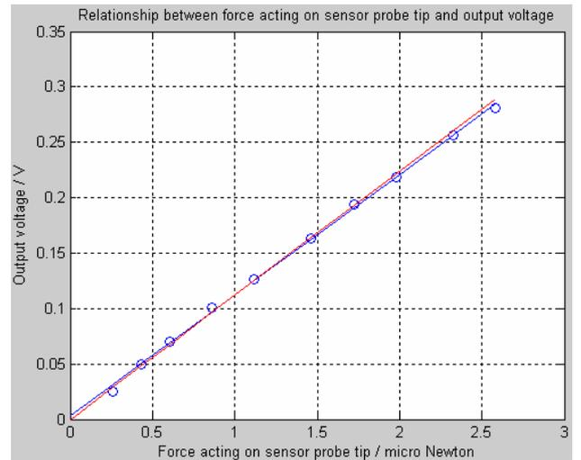
Fig. 6 The curve of relationship between the micro interactive force and output voltage of signal processing circuit.
