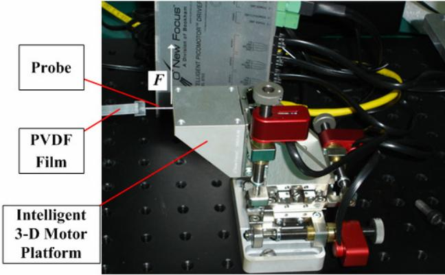
Fig. 4 The schematic diagram of calibration experiments.
