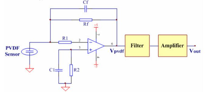
Fig. 2 The diagram of PVDF sensor signal processing circuit.
