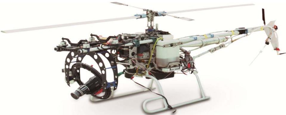
Fig. 2. SERVOHELI-40 small-size helicopter platform
