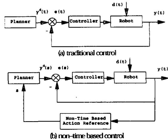
Figure 4. Comparison between traditional time-based and event-based planning and control.
