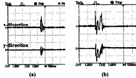
Figure 9. Experimental voltage output of the 2-D PVDF sensing system for a commercial probe manipulator. Shown are the 2-D sensor signals of the probe-tip impacting a substrate at (a)  $v=3000\mu\text{m}/\text{sec}$ , and (b)  $v=6000\mu\text{m}/\text{sec}$ .
