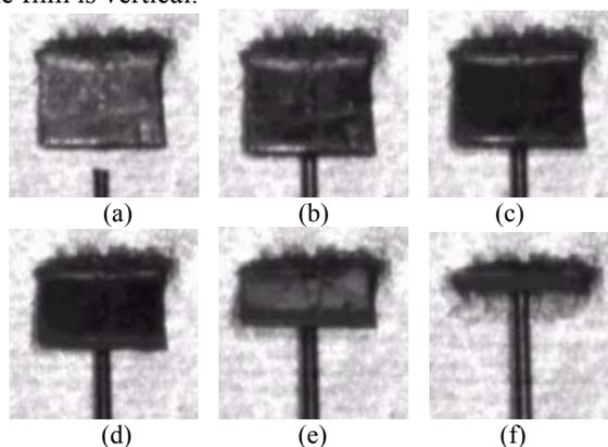
Fig. 5. Assembly of Micro Mirrors With Micro Force Sensor
