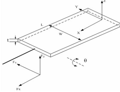
Fig. 1. Structure of PVDF Micro Force Sensor
