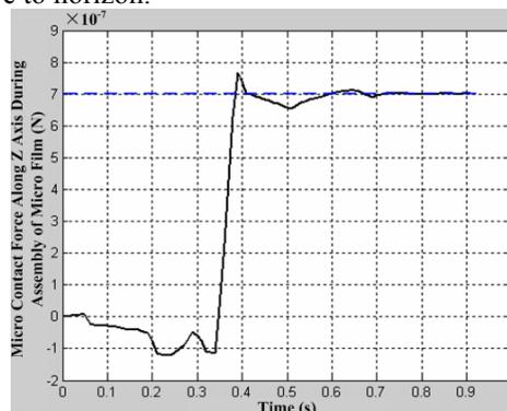
Fig. 6. Contact Force along Z Axis in Assembly of Micro Film
